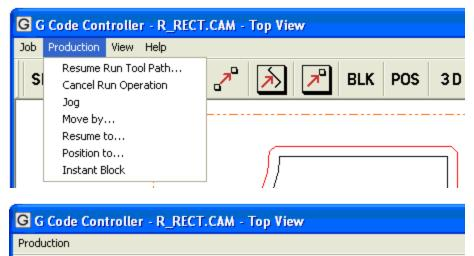
If a **Job** is currently in progress, either by **Apply**(ing) a resuming **Block** location from the **Simulator**, or **Suspend**(ing) from a **Production Run** dialog, then options to **Resume** or **Cancel** the **Job** also appear under the **Production** menu and in the **Toolbar**. (**Resume** appears in the **Toolbar** as a button entitled
