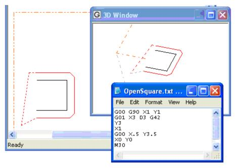
**Rapid Traverse** (G00) entering into and leaving a contour is automatically adjusted, as illustrated in the screen clip. (The part programmer should be aware that in some circumstances it is necessary to insert an intermediate rapid traverse movement to keep the automatically adjusted rapid path clear of the material).
