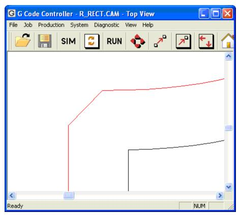
keyboard. Magnification is increased each time you press **Page Down**, and the **Scroll Bars** are automatically adjusted to according to the point that you had selected to appear in the center of the screen. Press **Page Down** successively to increase magnification (Zoom In). Press the **Page Up** key to decrease magnification (Zoom Out). The cursor position has no effect when pressing **Page Up** to Zoom Out.
