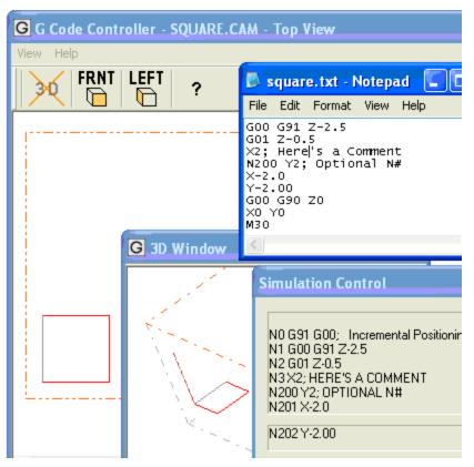
window shows the original text of the **Part Program** Blocks preceding the line assigned a number, N200 are automatically assigned and incremented. After N200, unassigned lines are assigned incrementally higher values.
