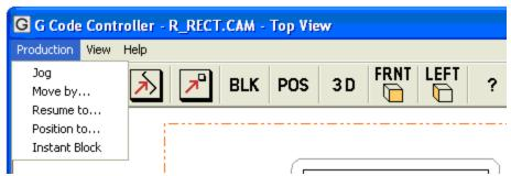
This illustration shows how the **Production** menu may appear after the **Run** (or **Dry Run**) **Tool Path** dialog has been opened. Manual motion dialogs are accessible, including **Resume to**, which provides assistance positioning the **Stages** to a resuming position along the tool path. Dialogs that affect initializing the **Machine Home** position: **Set Home** and **Limit Switch Seek**, are absent in this context.
