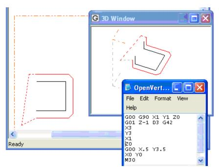
tion in the X-Y plane as it starts, as shown in the illustration. For closed contours the best offset path needed to cut the entire perimeter of the contour is used. The offset point into a closed contour is located at a point on the optimized tool path, also shown in the screen clip.
