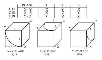
**Stage** position words are used to specify destination points according to the plane of operation. For the (G17) X-Y plane use X and Y, for the (G18) X-Z plane use X and Z, and for the (G19) Y-Z plane use Y and Z.
