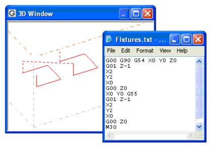
All absolute positions referenced in the part program represent distances from the current fixture offset position, otherwise known as **Program Zero**. The fixture offset position is specified as a distance from the **Machine Home** position, which is either automatically set after a **Limit Switch Seek** sequence, or reset by means of the **Production > Set Home** dialog (Refer to the section
