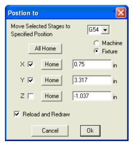
Unlike the **Move by** dialog, **Position to** requires position tracking to have been initialized via the a completed **Limit Switch Seek Sequence** or the **Set Home** control.
