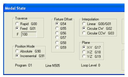
The **Modal State** display (split in the illustration to fit on the page) shows states of the machine that remain in effect as they are controlled by the part program. (Commands that set a machine state and remain in effect from **Block** to **Block** are called "Modal").
