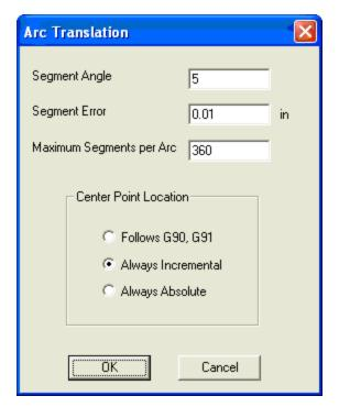
means of line segments situated end to end across the path of the true theoretical arc. As per the diagram on the next page, the **Segment Angle** is the maximum subtended angle for each line. In other words, as long as the geometry does not violate the **Segment Error**, or the **Maximum Segments per Arc**, the arc will be constructed in segments using **Segment Angle** or less.
