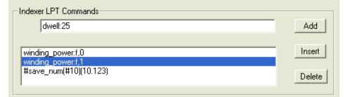
command. The **Add** button transfers the command that you had typed to the bottom of the list. Scroll bars automatically appear when the list grows larger than the display window. You can insert a command by highlighting the command before which you want the item inserted, and then snap **Insert**. Items can be deleted by highlighting the command you want removed and snapping **Delete**.
